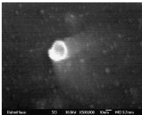
Fig. 8. FESEM images of palladium (Pd loading = 8000 pulses) deposited on silicon showing a 30 nm particle. Particles <5 nm are clearly evident.
